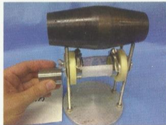
Fig. 1: The instrument used to produce excessive condensate
